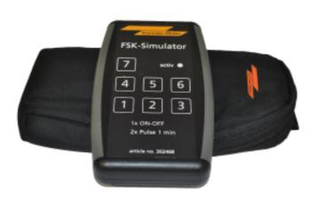
DIMENSIONS lenght: 90mm width: 150mm depth: 25mm
