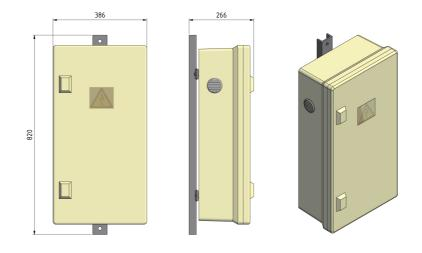
DIMENSIONS length: 820 mm width: 386 mm height: 266 mm
